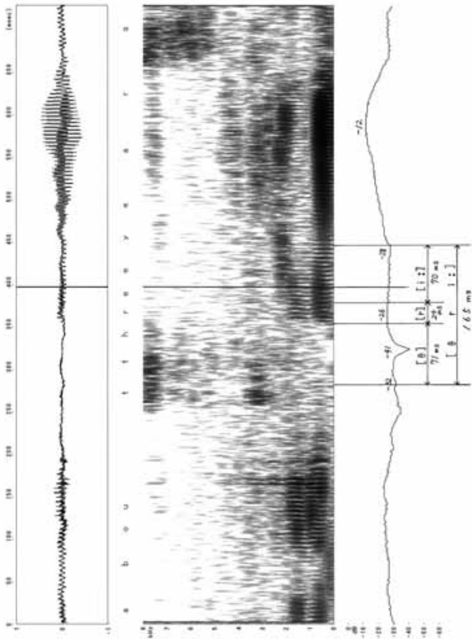
Figure 1 Waveform, Spectrogram, and Pressure Contour of “about three years”
